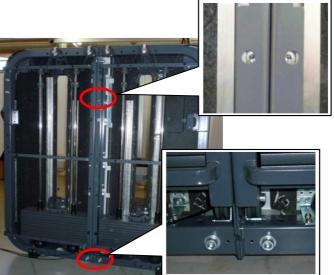
Insert the rear foot in the frame assembly, tighten with 2 screws (K) + 1 screw (J) + 2+2 washers + nut (F1), position and tighten the piston unit plate with 2 screws (F2)
