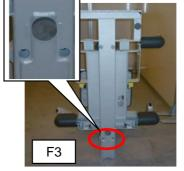
Turn the platform assembly by 90°, insert it in the frame assembly and tighten with 2+2 screws + 2+2 washers
