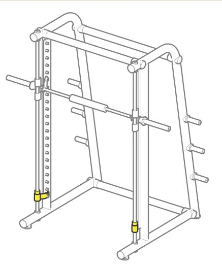
**Safety stops**: are positioned on the barbell support pins to set the lowest travel limit of the barbell.
