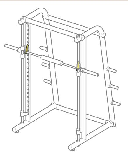
**Stop hooks**: are operated by the user with a twist of the wrist, to lock and release the barbell on the supports.
