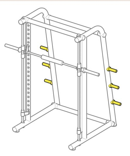
Weight plate storage posts: are used for holding the weight plates (not included) that are not needed for the exercise.
