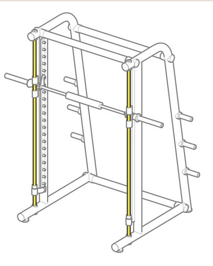
Barbell: moves up-and-down on the **guide rods** and provides the exercise workload. The weight plates can be positioned on its ends to increase the workload.
