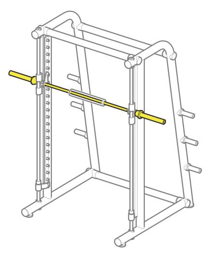
**Barbell**: moves up-and-down on the <u>guide rods</u> and provides the exercise workload. The weight plates can be positioned on its ends to increase the workload.
